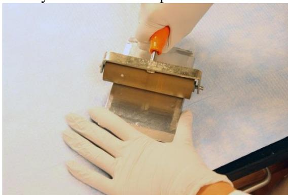
**Step 3:** Secure the outer edges of the plate by wrapping parafilm around the perimeter of the plate.
