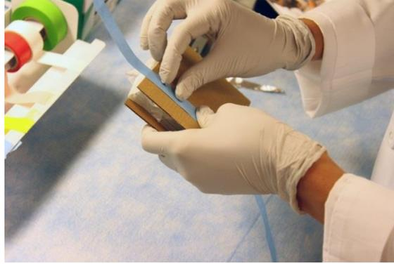
**Step 7:** Each plate must be secured in its own cardboard sandwich and sealed in individual bags.
